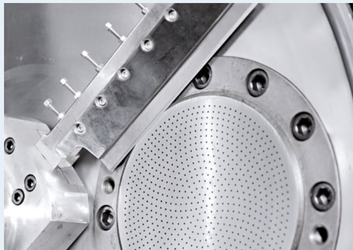
› KNIFE AND DIE PLATE OF STS Mc 11 TWO-STAGE COMPOUNDER
