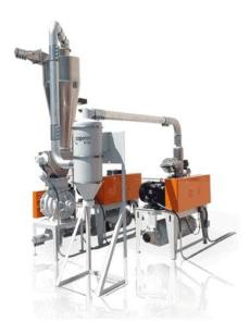
The Coperion K-Tron dual-blower Rail Unload System pneumatically transfers pellets, powder and granular materials from railcars at conveying rates in excess of 120,000 lbs/hr (54,430 kg/hr).
