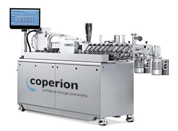
Making its debut in the USA is Coperion's newly redesigned ZSK 26 Mc<sup>18</sup> twin screw laboratory extruder with 25 mm screw diameter. It has an increased torque of 15 Nm/cm<sup>3</sup> and is capable of throughputs of up to 100% higher than its predecessor, but it also has all the advantages of the ZSK Mc<sup>18</sup> series.
