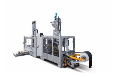
Coperion's intelligent FFS Packaging Machine IBP 250 with automated features provides accurate weighing, ideal dosing and hygienic packaging for crystalline, granular, beaded or flaked goods.
