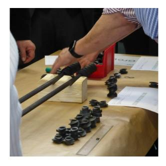
Participants practicing screw configuration by "threading" various screw elements (conveying, mixing, shearing) onto the screw shafts.
