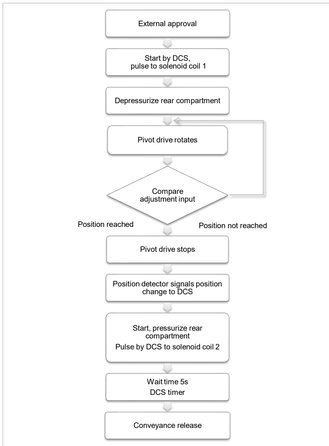
Fig. 5.5: Flow chart 2: Switching a WHK-W with a FESTO controller
