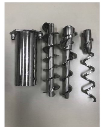
Single Screw with and without overflight to avoid product in the bowl
