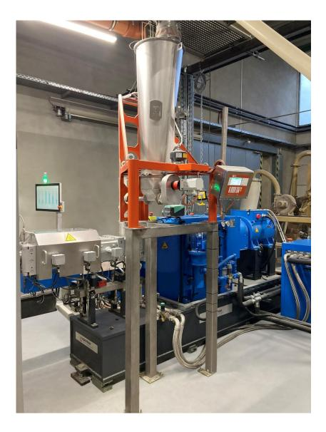
The Düngemittelwerk Coswig company has expanded production of fertilizer spikes with a Coperion ZSK extruder, equipped with a ProRate PLUS-MT twin screw feeder.
