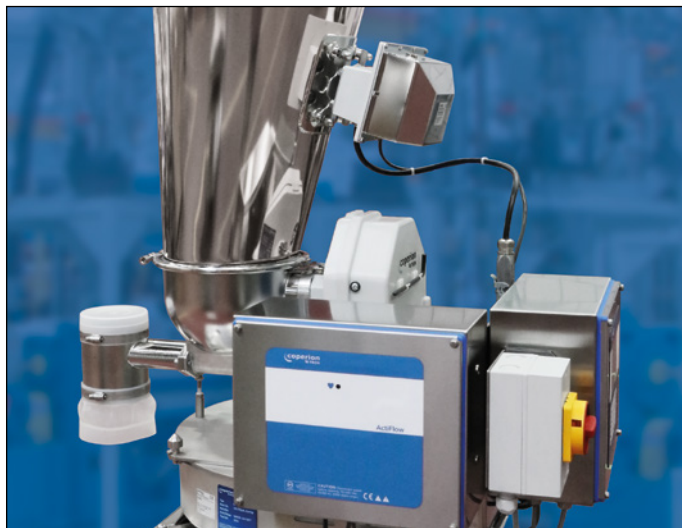
ActiFlow is mounted outside the product zone and has minimal space requirements
