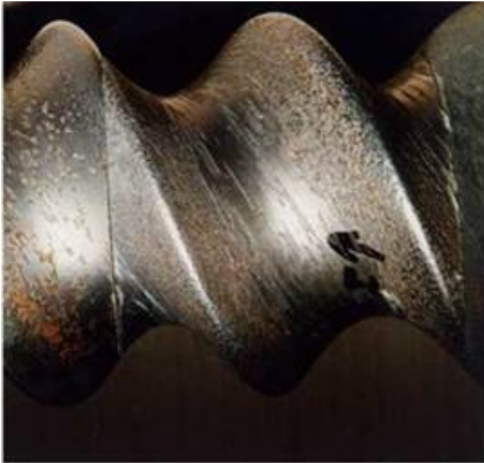
Combination of abrasive wear and corrosion
