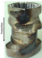
Excessive wear due to abrasive materials
