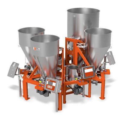
The ProRate PLUS feeder line features a space-saving trapezoidal shape which allows up to six feeders to be easily grouped around an extruder inlet within a 1.5 meter [5 ft] radius.
