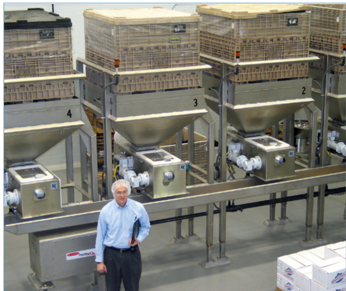
Smart Weigh Belt Feeders in a snack blend process
