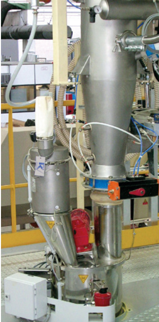
Feeder refill via vacuum receiver
