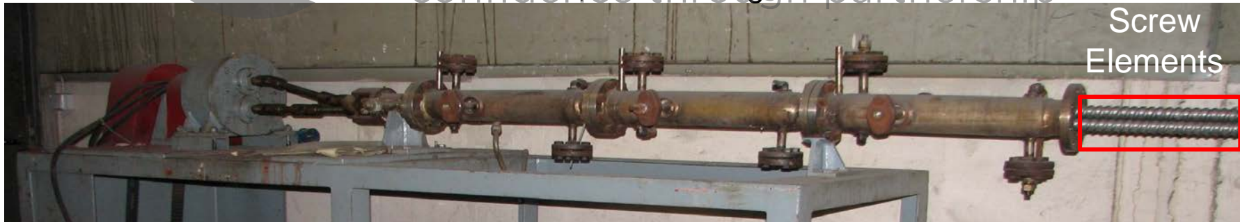
Lab Extruder 1940's, R. Erdmenger
