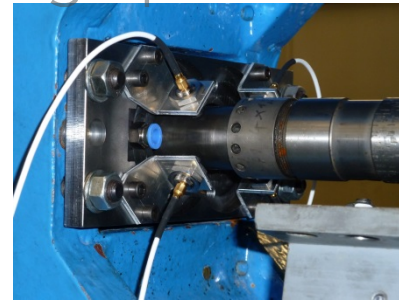
Measurement of mechanical deflection in vertical and horizontal direction
