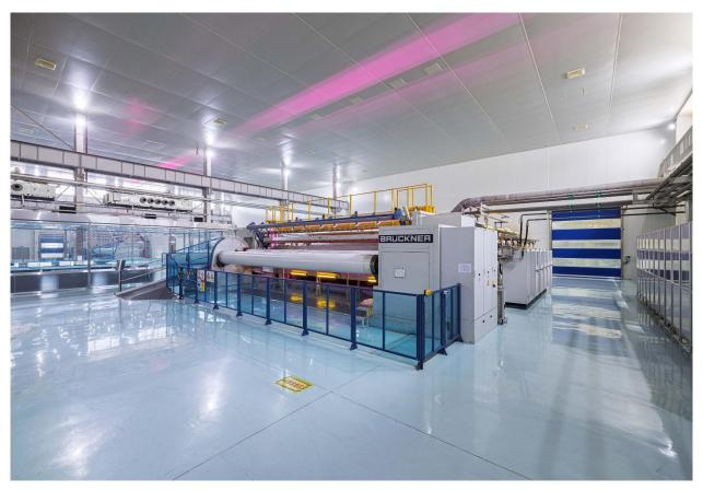
For its plastic film stretching lines Brückner Maschinenbau relies on Coperion ZSK extruders, which melt the raw material.
