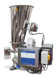
Hall 14 | Booth B19 — Coperion K-Tron T35 twin screw feeder shown here with ActiFlow bulk solid activator and KCM-III Controller.
