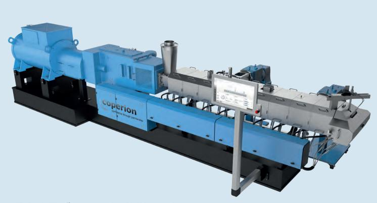
>The Coperion ZSK Mc<sup>18</sup> twin screw extruder, with its high torque and gentle processing, is especially well-suited for manufacturing high-quality recycling compounds.
