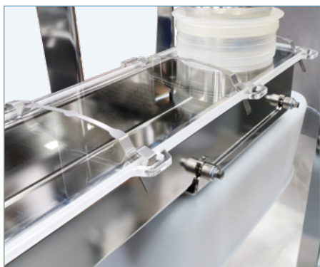
Special quick-release clamps hold the cover on the tray.
