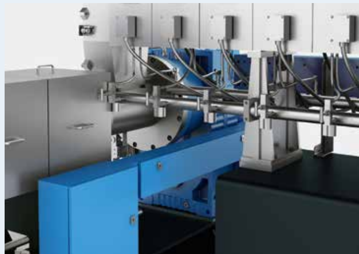
› TRANSFER FROM TWIN SCREW TO SINGLE SCREW PROCESS SECTION
