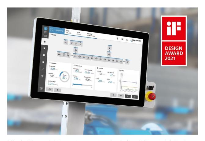
Using the CSpro control, the operator can easily and precisely control the extruder's functions. The risk of possible operator error is markedly reduced, thus increasing the ZSK extrusion equipment's efficiency.
