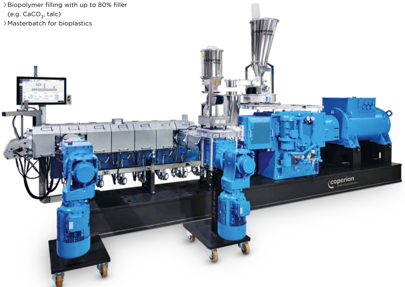
› ZSK TWIN SCREW EXTRUDER WITH HIGH-ACCURACY FEEDERS, ZS-B SIDE FEEDER AND ZS-EG SIDE DEVOLATILIZATION
