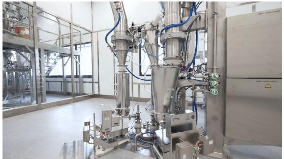
Coperion K-Tron pharmaceutical feeders are an integral part of the Pfizer high containment automated production facility in Germany.
