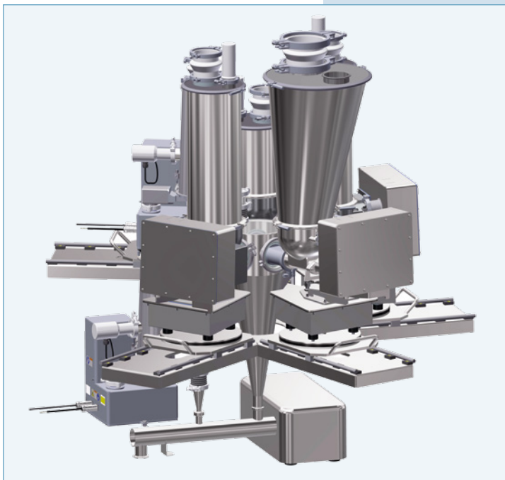
Five K3-PH feeders on special slide mounts clustered over a continuous mixer inlet.
