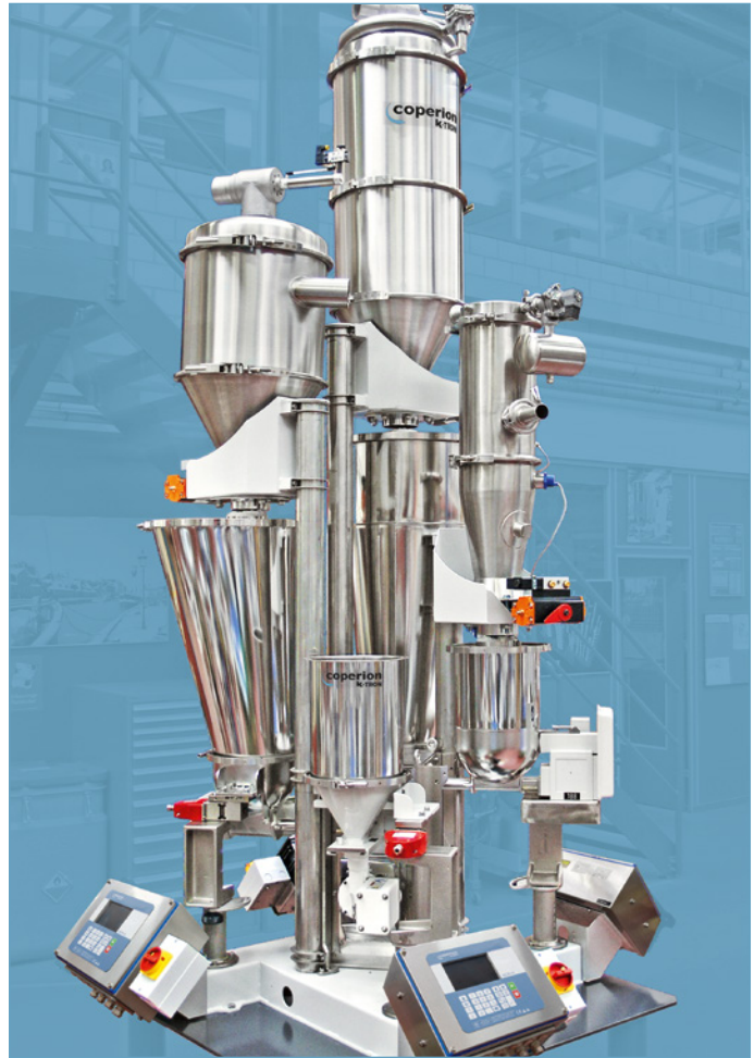
Coperion K-Tron receivers refilling Coperion K-Tron loss-in-weight feeders
