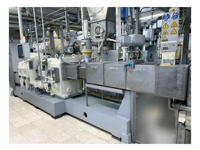
Within a few weeks, Coperion successfully implemented a comprehensive control system upgrade, allowing Tetra's ZSK twin screw extruder to once again produce fish feed pellets at full productivity and efficiency.
