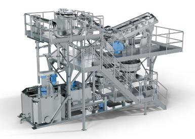
The Hydrocyclone Separation Stage uses centrifugal forces and turbowasher technology to accurately separate and purify plastic materials, enhancing recycling efficiency and material quality.
